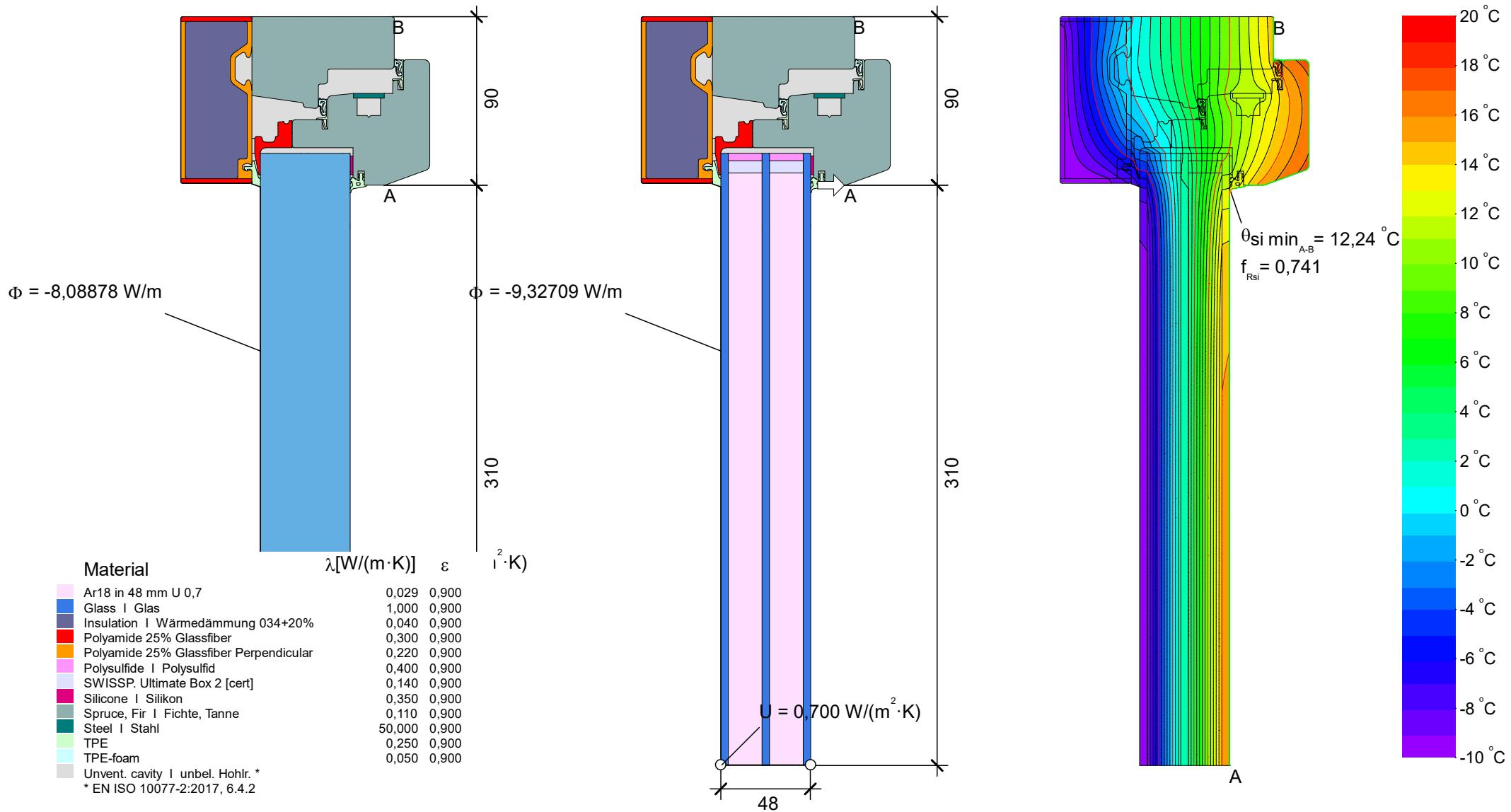
$$U_{f,A,B} = \frac{\frac{\Phi}{\Delta T} - U_p \cdot b_p}{b_f} = \frac{\frac{8,089}{30,000} - 0,649 \cdot 0,310}{0,090} = 0,761 \text{ W/(m}^2\text{·K)}$$
