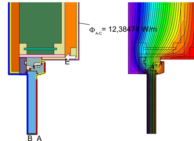
$$\psi_{A-E-C,*} = \frac{\Phi}{\Delta T} - \frac{\Phi_1}{\Delta T} - U_2 \cdot b_2 = \frac{12,385}{30,000} - \frac{8,089}{30,000} - 0,131 \cdot 1,010 = 0,011 \text{ W/(m·K)}$$
