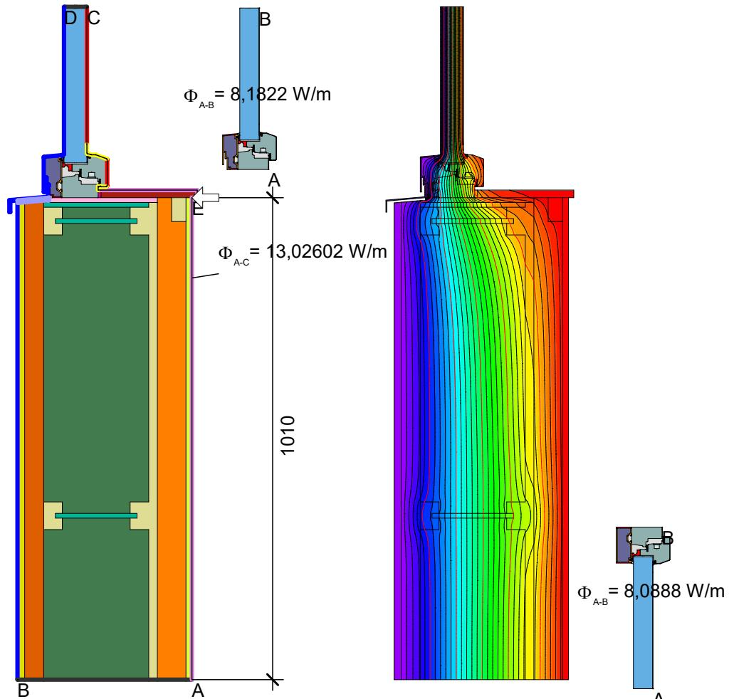
$$\psi_{A-E-C,*} = \frac{\Phi}{\Delta T} - U_1 \cdot b_1 - \frac{\Phi_2}{\Delta T} = \frac{13,026}{30,000} - 0,131 \cdot 1,010 - \frac{8,182}{30,000} = 0,029 \text{ W/(m·K)}$$
