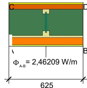
$$U_{eq A-B} = \frac{\Phi}{\Delta T \cdot b} = \frac{2,462}{30,000 \cdot 0,625} = 0,131 \text{ W/(m}^2 \cdot \text{K)}$$
