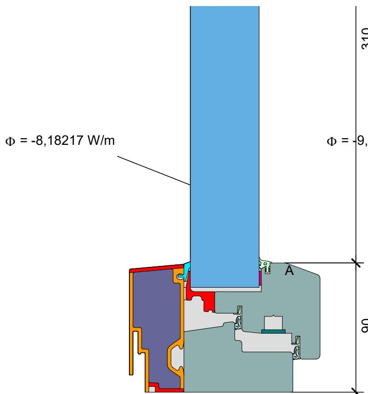
$$U_{f,A,B} = \frac{\frac{\Phi}{\Delta T} - U_p \cdot b_p}{b_f} = \frac{\frac{8,182}{30,000} - 0,649 \cdot 0,310}{0,090} = 0,796 \text{ W/(m}^2\text{·K)}$$
